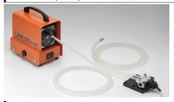
The vacuum pump set for fiber holder and device holder. Put a release valve on the bread board when use
