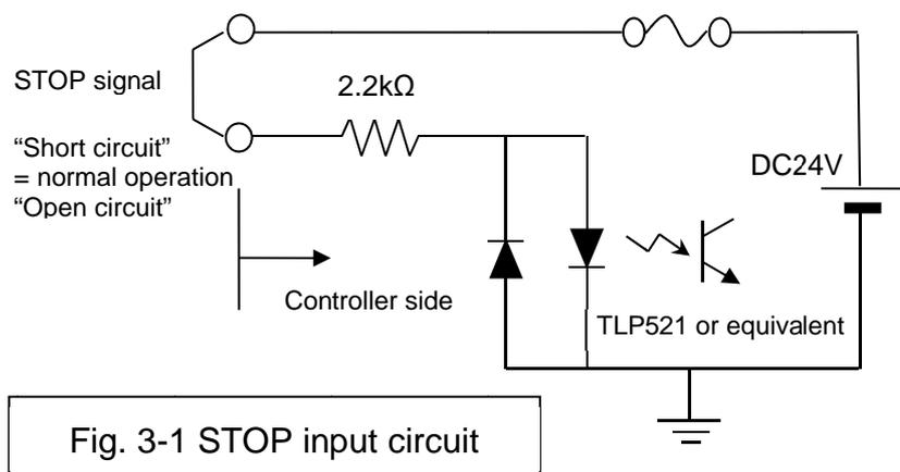
**(Caution)** Turn off the controller power, while connecting the stop signal input.
