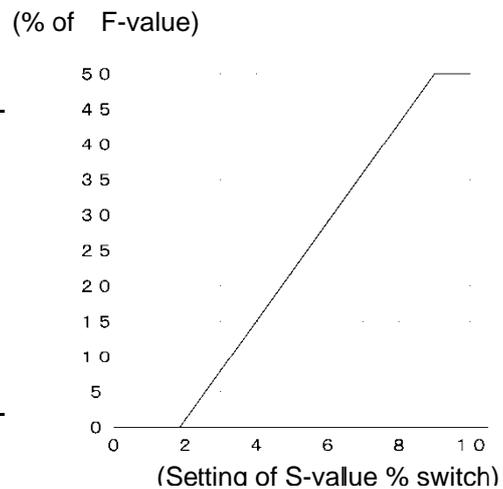
Fig. 3-2-3 Relation of “S-value % switch” setting and % of F-value
