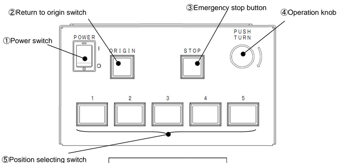
Fig. 2-1-1 Front Panel
