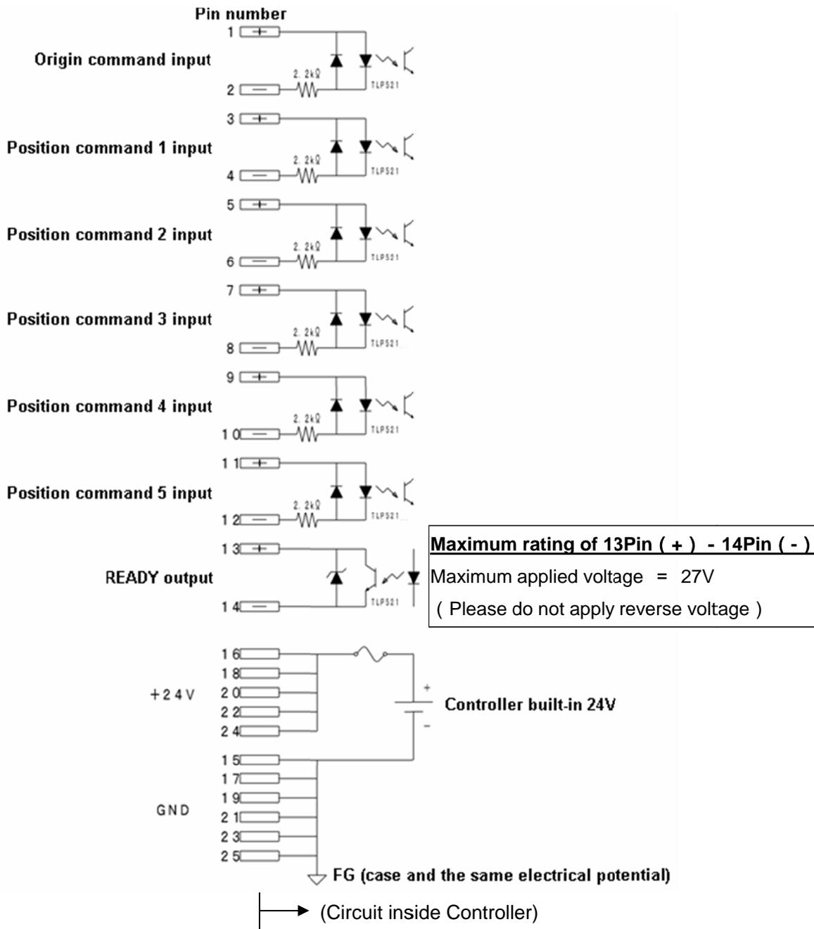
Fig. 3-4-3 I/O connector signal
