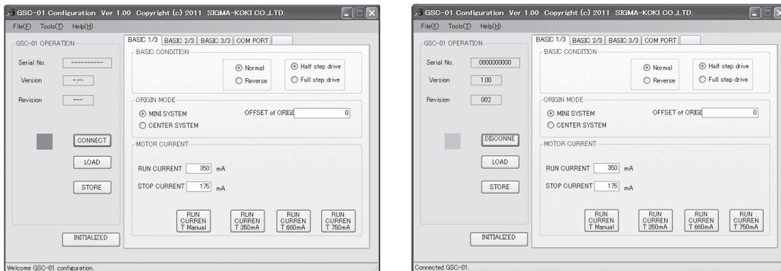
If the communications have been established successfully, the above screen is displayed, the indicator turns green is displayed. If an error is displayed, you must check the connection and the baud rate setting again.
