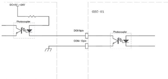
Fig.7-3 I/O OUT(DO0) connection example
