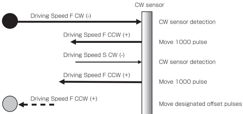
If no offset is specified, sets the home position after 1000pulse movement without doing it.
