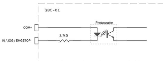
Fig. 7-1 I/O Input (DIO-3, JOG, EMGSTOP) Circuit
