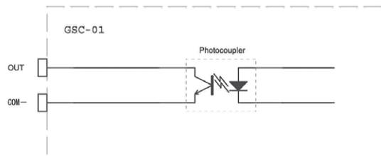
Fig. 7-2 I/O Output (DO0-3) Circuit
