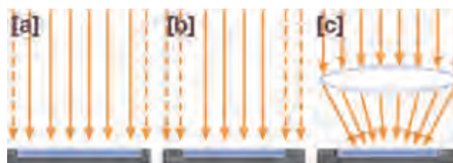
Figure 5: Cross sectional view of pixels with different fill factors (blue area corresponds to light sensitive area) and the light rays which impinge on them (orange arrows). Dashed light rays indicate that this light does not contribute to the signal: [a] pixel with 75 % fill factor, [b] pixel with 50 % fill factor and [c] pixel with 50 % fill factor plus micro lens on top.
