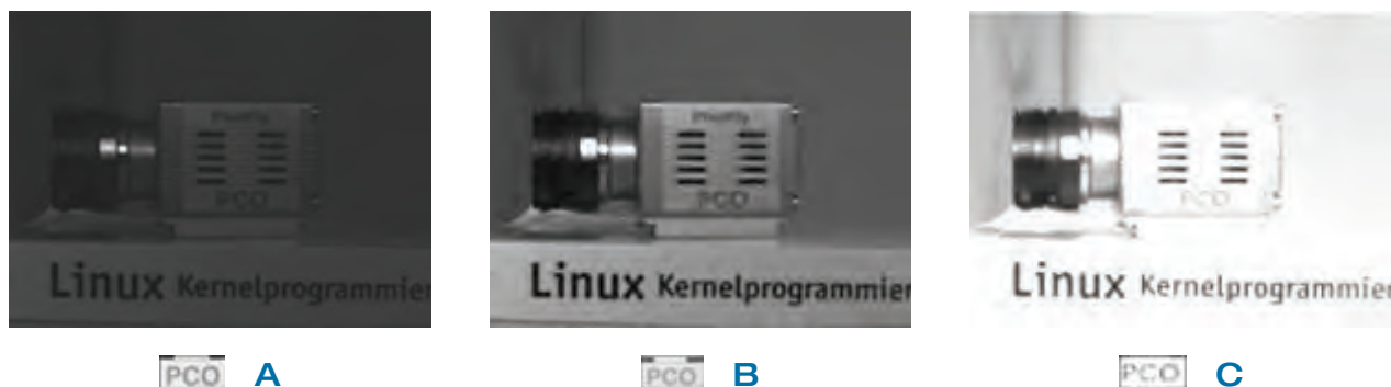
Figure 2: The same series of images with increasing binning from (a) to (c) (like above), only the images with lower resolution have been blown up in size, show the loss in spatial resolution. The detail images showing the letters “PCO” have been further processed in terms of brightness and contrast to elucidate the loss of spatial resolution by binning.
