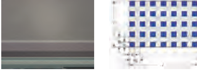
Figure 2: a) A macro image of a CCD image sensor showing the pixels at the edge of the imaging area, b) illustration of an image sensor with characteristic geometrical parameters: x , y - horizontal, vertical dimensions, p_x , p_y - horizontal, vertical pixel pitch, b_x , b_y - horizontal, vertical pixel dimensions
