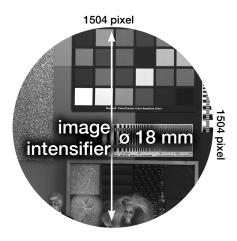
The projected image circle is completely covered by  $1504 \times 1504 \times 6.5 \mu m$  pixels of the sCMOS detector. There is no "waste" of valuable intensifier area. As a consequence, the four corners of the sCMOS sensor remain black.
