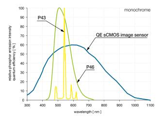
This chart describes the spectral situation for the internal imaging of the image intensifier's phosphor output screen to the sCMOS sensor of the camera detector module. This imaging is done by the highly efficient tandem lens system.
