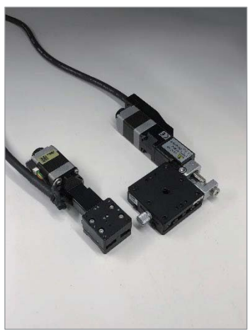
Comparison of TSD-401S + SGSP-13ACTB0(right) and OSCM25-10X(left)
