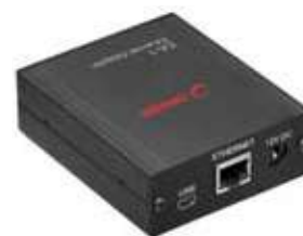
Mini-USB connector; Ethernet RJ45 connector; 12V power connector
