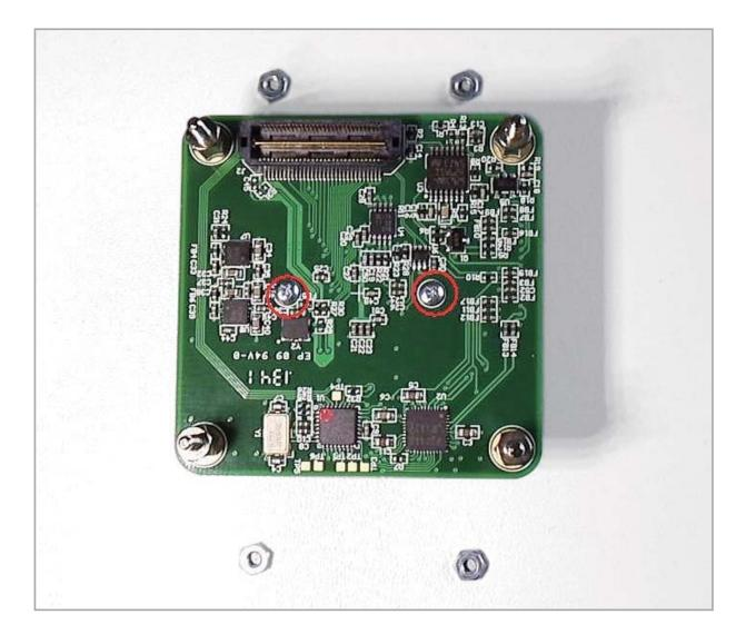
• Place the lens holder over the sensor on the front of the PCB. Turn the PCB over. Using the two fixing screws provided, affix the lens holder from the back of the PCB. The red circles above show the placement of the fixing screws.
