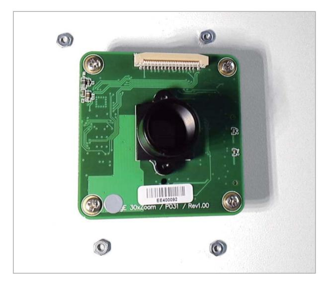
• With the lens holder now mounted to the front of the PCB, replace the back PCB to its original position ensuring that the inter PCB connector is closed.
