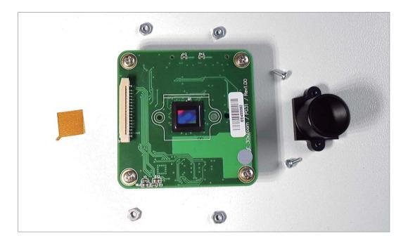
Remove protective foil from sensor
