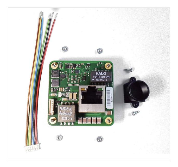
• Unscrew the four nuts from the camera back.
