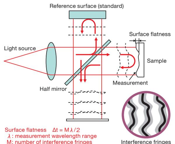
To measure surface accuracy with an interferometer, install a sample in one optical path, and superimpose the wavefront reflected by the measuring surface with the plane wave reflected by the reference surface. Interference fringes generated at this time are folded, reflecting the shape of the measuring surface.
