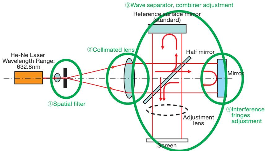
When installing components, firmly fasten various joints or clamps so that holders do not move. Such parts include the coarse/fine switching clamps for elevation and azimuth of a mirror holder, or clamp of a post holder, the on/off of the lever of a magnet base. If joints or clamps are not fastened, vibrations tend to occur, making stable observation of interference fringes difficult.
