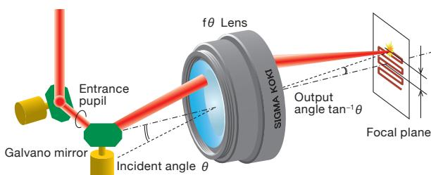
By using the f theta lens, it is possible to move a laser light spot in constant speed linear motion on the focal plane by scanning the mirrors such as galvanometer scanner mirrors.
