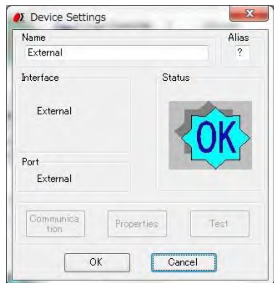
In the case of an external device Communication, Properties, and Test button are not used.
