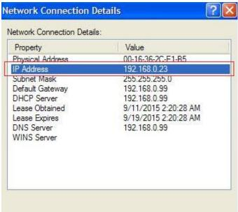
If the segment of the PC's IP address (192.168.0.  $\Box$ ) is the same as the controller, there is no need to change it, but if it is different, change it.
