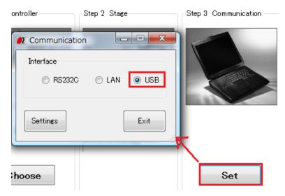
After completing communication setup, perform communication test in step 4. In the communication test, if you click "Connect" button and "Result" becomes "OK", connection is completed.
