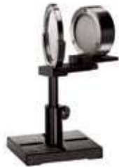
Beam splitter installed – reflected beam on sensor
