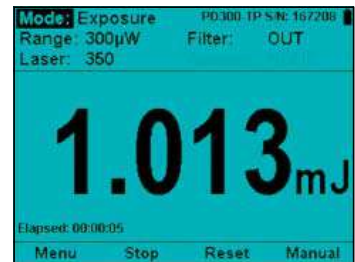
Exposure measurement (energy summing) with photodiode sensor.
