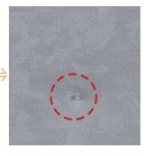
The diffused light from the Dome Light negates differences in surface tone, making it possible to notice faults.
