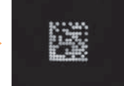
It is possible to determine the 2-D code by evenly illuminating the surface.
