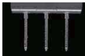
Illumination from the front of the workpiece allows you to observe the surface state of the connector.
