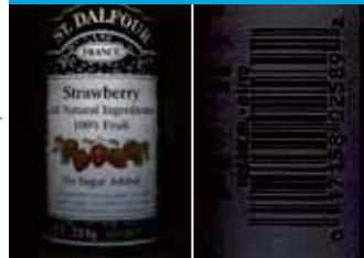
Shutter speed: 1/10,000 Shutter speed: 1/18,000 Amount of light: 100% intensity Continuous lighting: 100% intensity
