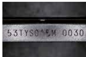
It is difficult to observe the engraved characters due to uneven illumination.
