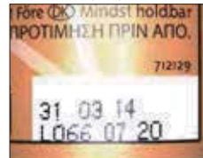
Illuminated light converges in the center, making stable inspection difficult.
