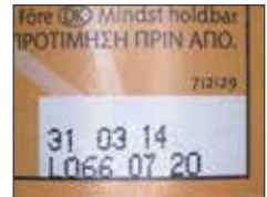
The whole thing is evenly and brightly illuminated, making it possible to take an image of the label text.
