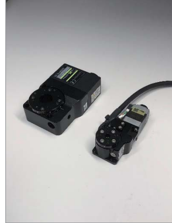
Comparison of OSCM-25YAW (right) and OSMS-40YAW (left)
