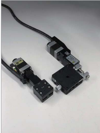
Comparison of TSD-401S + SGSP-13ACTB0(right) and OSCM25-10X(left)
