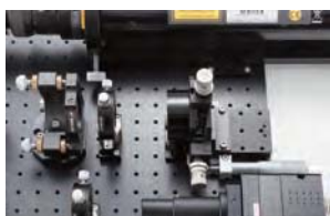
Concave sample and achromatic lens
