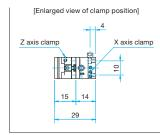
Wrench size for adjustment XY axes=3mm, Wrench size for clamp common to XYZ axes=0.89mm Pan head screw M2×6...3 screws, One 3mm hex wrench with knob, One 0.89mm hex wrench **TASB-255**
