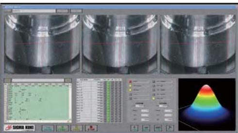
Software with an image impose function added to the alignment software ASS-02.
