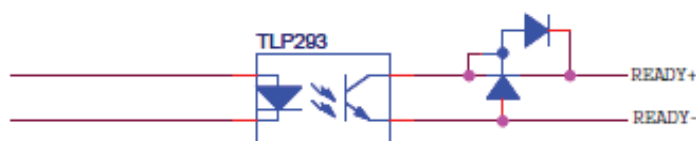
Fig4-2 Output circuits (READY)
