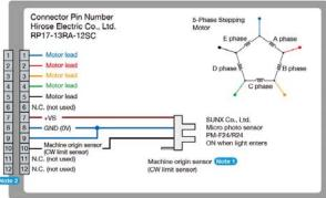
Note 1 When a travel command in the "+" direction is issued, the mounting table rotates to ∞ in the CCW (counterclockwise) direction viewed from the top surface, but it is stopped by the machine origin sensor (CW limit sensor) in the CW (clockwise) direction. Detect the machine origin using the method (MINI system) that detects the origin with a machine origin sensor (CW limit sensor).
