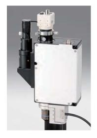
The Through The Lens auto focus method incorporates the focusing system into the microscope body, directing the focus laser through the objective lens. The reflected beam returns through the objective lens and id focused onto the focus sensor.
