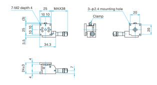
MLT63-40 Hexagon socket head cap screw (stainless steel construction) M3×8...3 screws
